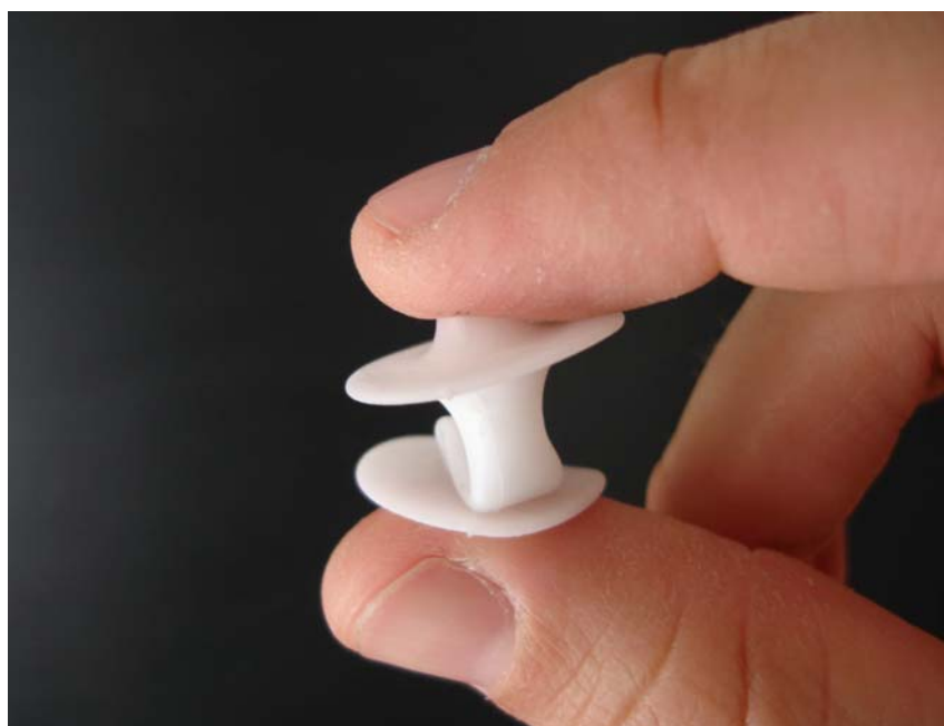
Figure 5. Demonstration of the softness and deformability of the Enshur Insert
